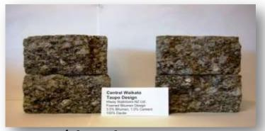
"Care should be taken to ensure that cracking is not a primary mode of failure by limiting the application of cementitious additives".
