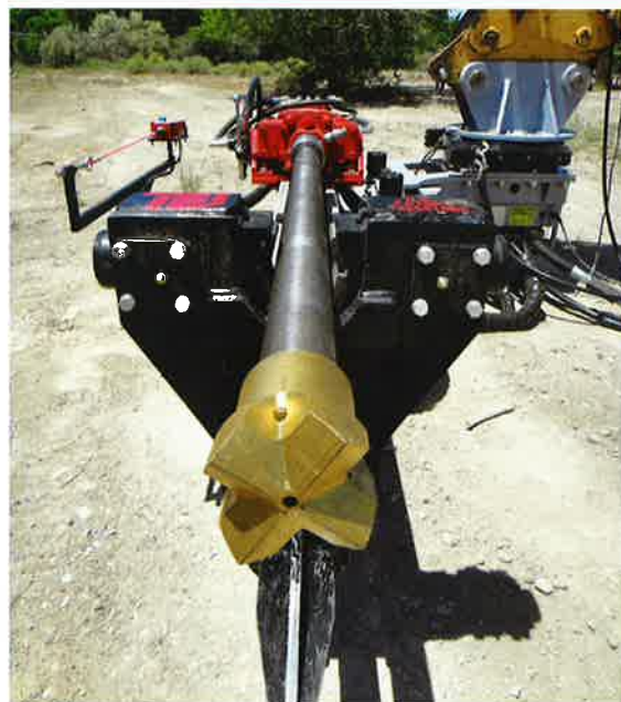
A Williams 76mm hollow bar with 133mm bit
